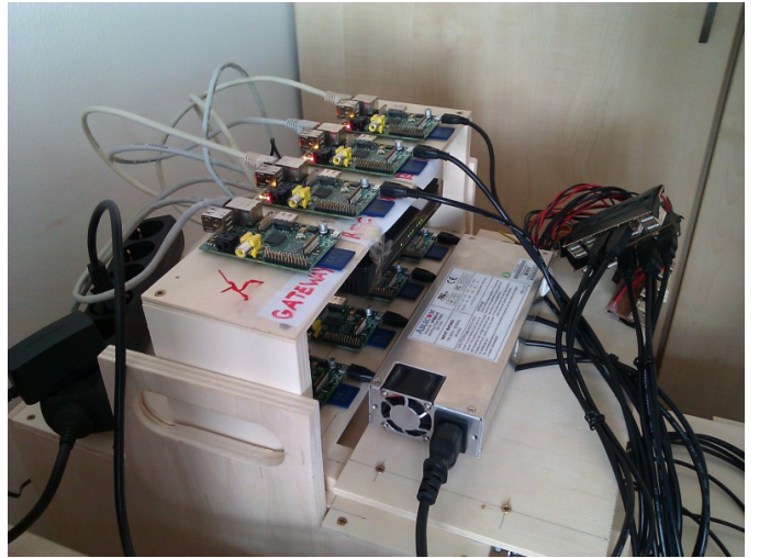
Fig. 7. Bobino, the Raspberry Pi cluster used in our experiments
